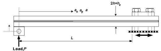
As clamping fixtures were not standard, the ELS method was revised to calibrate the clamp
