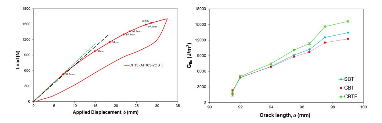
Even stronger rising mode II R-curve measured but not reaching a steady-state. Some indication of specimen damage around clamping support.
